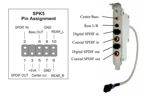
*Note:* Some 5.1 speakers have different center/base assignment. Please use the C-media Multi-Channel Audio demo software to check if sounds coming from the center/base speaker are correct. Adjust JP30 accordingly if not.
